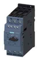
Circuit breaker size S2 for motor protection, CLASS 10 A-release 62...73 A N-release 949 A screw terminal Standard switching capacity with transverse auxiliary switches 1 NO+1 NC
