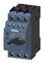
Circuit breaker size S0 for motor protection, CLASS 10 A-release 18...25 A N-release 325 A Screw terminal Standard switching capacity with transverse auxiliary switches 1 NO+1 NC
