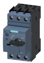
Circuit breaker size S0 for motor protection, CLASS 10 A-release 0.9...1.25 A N-release 16 A screw terminal Standard switching capacity
