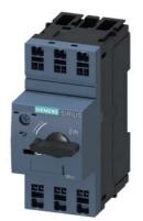
Circuit breaker size S00 for motor protection, CLASS 10 A-release 5.5...8 A N-release 104 A Spring-type terminal Standard switching capacity
