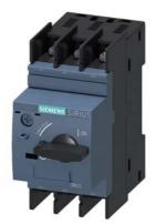
Circuit breaker size S00 for motor protection, CLASS 10 A-release 3.5...5 A N release 65 A ring cable lug connection Standard switching capacity
