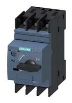
Circuit breaker size S00 for motor protection, CLASS 10 A-release 2.2...3.2 A N release 42 A ring cable lug connection Standard switching capacity
