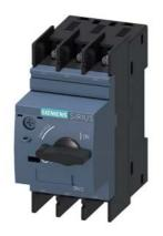
Circuit breaker size S00 for motor protection, CLASS 10 A-release 1.8...2.5 A N-release 33 A ring cable lug connection Standard switching capacity
