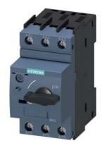
Circuit breaker size S00 for motor protection, CLASS 10 A-release 1.8...2.5 A N-release 33 A screw terminal Standard switching capacity
