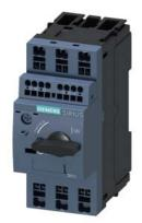
Circuit breaker size S00 for motor protection, CLASS 10 A-release 0.14...0.2 A N-release 2.6 A Spring-type terminal Standard switching capacity with transverse auxiliary switches 1 NO+1 NC
