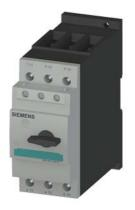
Circuit breaker size S2 for motor protection, Class 10 A-release 36...45 A Short-circuit release 540 A 1 NO + 1 NC transverse Screw terminal Standard switching capacity !!! Phased-out product !!! Successor is SIRIUS 3RV2 Preferred successor type is >>3RV2031-4VA15<<
