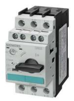
Circuit breaker size S0 for motor protection CLASS 10 A-release 14...20 A Short-circuit release 260 A Screw terminal Standard switching capacity with transverse auxiliary switch 1 NO+1 NC !!! Phased-out product !!! Successor is SIRIUS 3RV2 Preferred successor type is >>3RV2021-4BA15<<
