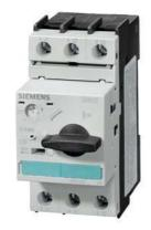
Circuit breaker size S0 for motor protection CLASS 10 A-release 2.8...4 A Short-circuit release 52 A Screw terminal Standard switching capacity !!! Phased-out product !!! Successor is SIRIUS 3RV2 Preferred successor type is >>3RV2011-1EA10<<
