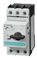
Circuit breaker size S0 for motor protection CLASS 10 A-release 2.2...3.2 A Short-circuit release 42 A Screw terminal Standard switching capacity !!! Phased-out product !!! Successor is SIRIUS 3RV2 Preferred successor type is >>3RV2011-1DA10<<
