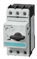
Circuit breaker size S0 for motor protection CLASS 10 A-release 0.55...0.80 A Short-circuit release 10 A Screw terminal Standard switching capacity !!! Phased-out product !!! Successor is SIRIUS 3RV2 Preferred successor type is >>3RV2011-0HA10<<
